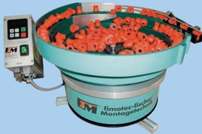
Vibration-feeding systems series VZ-AS with aluminium-step-shaped vibration bowls of 400 mm up to 860 mm diameter, coated with ear-proof polyurethane.
